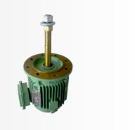
All fan motors are water-proof and totally enclosed (TEAO). Cooling tower motors are extended shaft flange mounted frame with weather proof IP55 Class F insulation.
